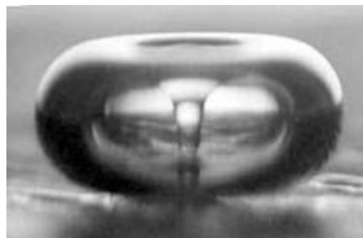
High speed jet Figure 2. Asymmetric bubble collapse
